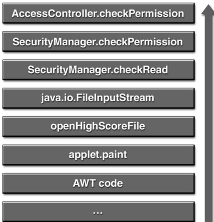
Figure 6.2. Stack frame execution context
