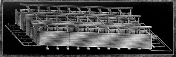
Fig. 34. Vertical Pipe Heating Apparatus for Dry Kilns; may be used in Connection with either Live or Exhaust Steam for High or Low Temperatures.
