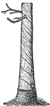
Fig. 15. Spiral Grain. Season checks, after removal of bark, indicate the direction of the fibres or grain of the wood.
