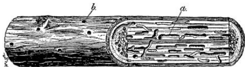
Fig. 27. Work of Powder Post Beetle, Sinoxylon basillare , in Hickory Pole. a , character of work by larvae; b , exit holes made by emerging broods.
