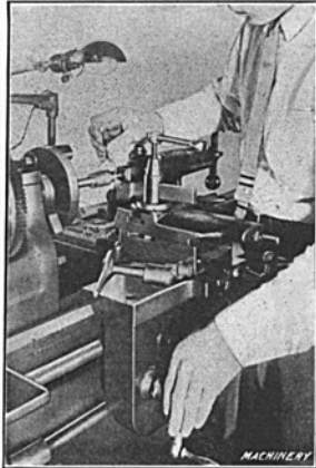
Fig. 10. Views showing how the Cross-slide and Carriage are Manipulated by Hand when Starting a Cut— View to Left, Feeding Tool Laterally; View to Right, Feeding Tool in a Lengthwise Direction
