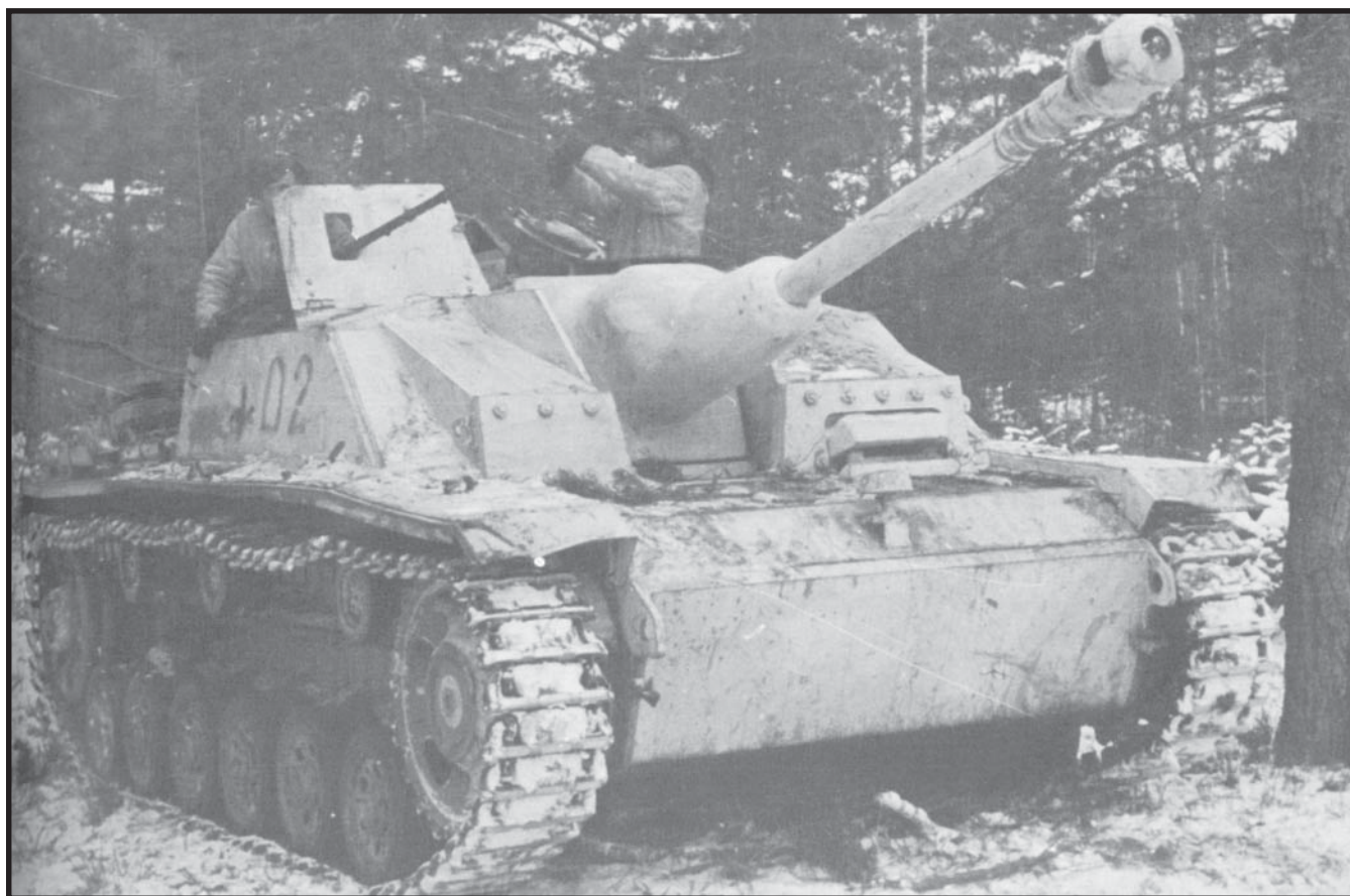
A Stuh 42 self-propelled gun in winter camo. Its 105mm gun provided heavy fire support for advancing infantry.
