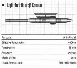
The Light Anti-aircraft Cannon is a high velocity, small-caliber weapon with an extremely high rate of fire, allowing it to fill a large area with deadly projectiles. An electric auto-loader brings fresh armmunition rounds, often caseless, from a magazine. It is usually linked to an air defense sensor system to increase its accuracy.
