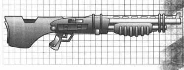
This style of shotgun contains several rounds in a tube magazine that is mounted underneath the barrel. A slide that forms the front handgrip is wrapped around the magazine and operates the feeding mechanism, which yanks a round from the chamber when the slide is pulled back. When the slide is brought back forward, a fresh round is pulled from the magazine and fed into the chamber. Pump-action shotguns are very common weapons, used by civilians, law enforcement and military personnel alike.
