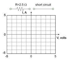
**Problem 2.4.** Given *v-i* characteristics of a resistance determine the corresponding conductance. Show units.
