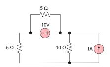
**Problem 3.70.** Determine the unknown current *I* in the circuit (solve by superposition).
