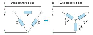
Fig. 11.27. Delta-connected load versus ad.
