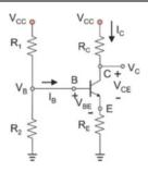
$$V_C = V_{CC} - \beta R_C I_B, I_B = \frac{V_{TH} - 0.7 \text{ V}}{R_{TH} + (\beta + 1)R_E}$$
