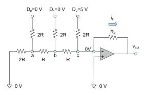
**Problem 5.46.** By solving the amplifier circuit shown in the following figure, determine its output voltage in terms of resistances R,  $R_{\rm F}$ , given the input voltages  $D_0=0$  V,  $D_1=5$  V,  $D_2=0$  V.
