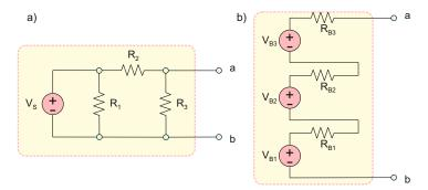
Fig. 4.13. Two active linear networks.
