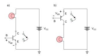
Fig. 17.27. Negative-side and positive-side BJT switches.
