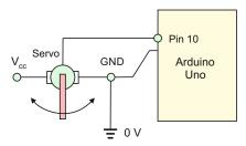
Fig. 15.16. Attaching a servomotor to the Arduino Uno.
