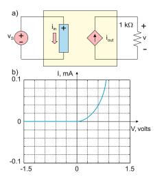
A nonlinear passive circuit element is shown by a rectangle. Element's polarity (direction of current inflow for passive reference configuration) of the element is labeled by a sign plus. The v-i characteristic of the element is also shown in the figure. The independent voltage source is given by  $v_{\rm S}=0.6\,$  V; the short-circuit current gain of the dependent source is  $100\,$  A/A.
