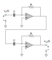
**Problem 6.49.** For the circuit shown in the following figure, express the output voltage,  $v_{\text{out}}(t)$ , as a function of time in terms of the input voltage,  $v_{\text{in}}(t)$ , and circuit parameters R, C. Assume ideal amplifiers.
