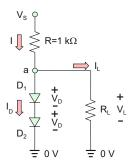
Fig. 16.18. Diode voltage reference for the load resistor  $R_{\rm L}$ .
