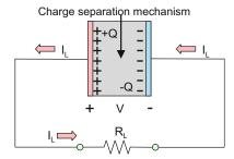
Fig. 2.26. Power source schematically represented as a capacitor continuously charged by a charge separation mechanism—the *charge pump*.
