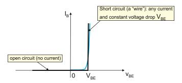
Fig. 17.13. Large-signal DC circuit model of the EBJ.
