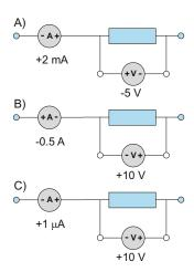
Based on voltage and current measurements, determine if the element is a resistance or a current source. Then, find the power delivered to the circuit element or taken from it in every case.
