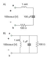
**Problem 11.21.** Determine the average power delivered to the load circuit shown in the figure below. The AC signal frequency is 10<sup>6</sup> Hz.
