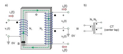
Fig. 12.12. Center-tapped transformer intended for single-ended to differential signal transformation (differential transformer) and the corresponding circuit symbol.
