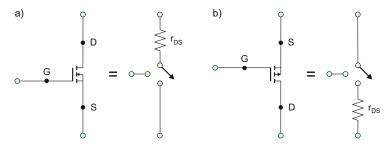
Fig. 18.19. MOSFET resistor-switch model in the triode region.
