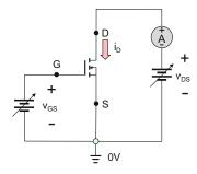
**Problem 18.31.** For the circuit shown in the figure that follows, determine the region of MOSFET operation as well as the drain current  $i_D$  for each set of conditions given. Assume  $k_p = 100 \text{ mA/V}^2$  and  $V_{Th} = -2 \text{ V}$ .
