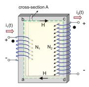
Fig. 12.2. Ampere's law for a transformer.
