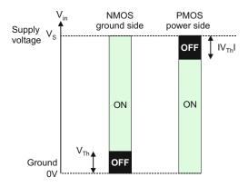
Fig. 13.4. Switching diagram for two MOSFET transistors.
