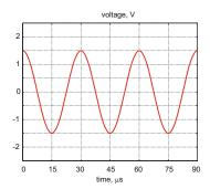
**Problem 14.41.** Determine frequency in Hz, angular frequency in rad/s, and amplitude of the harmonic voltage signal shown in the following figure.
