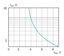
**Problem 18.36.** The datasheet for an IRF510 enhanced-mode n-channel power MOSFET from Fairchild reports the average drain-source *on-state* resistance  $r_{\rm DS} = v_{\rm DS}/i_{\rm D} = 0.4~\Omega$  for  $i_{\rm D} = 3.4~{\rm A}$  and  $v_{\rm GS} = 10~{\rm V}$ . Assuming threshold voltage to be 2.0 V, sketch  $r_{\rm DS}$  as a function of  $v_{\rm GS}$  to scale.
