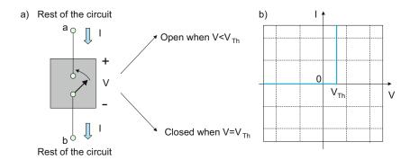
Fig. 2.14. (a) Two-terminal unidirectional threshold switch and (b) its ideal *v-i* characteristic.
