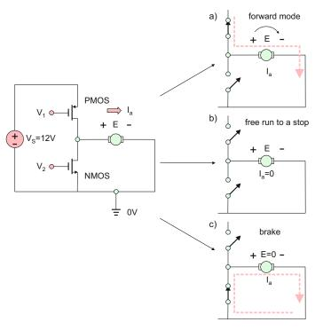
Fig. 13.13. Half H-bridge transistor switch with three motor functions.
