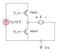
**Problem 13.20.** In the half H-bridge circuit shown in the figure to the previous problem, the control voltages  $V_1$ ,  $V_2$  are either 0 V or 12 V. If we denote the 0-V control voltage by 0 (low) and the 12-V control voltage by 1 (high), all possible combinations of the control voltages are covered by the table that follows (the table in fact lists all *binary numbers* from 0 to 3). Fill out the table using four states:
