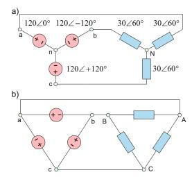
**Problem 11.53.** A three-phase balanced deltadelta system is shown in the figure that follows. Its wye-wye equivalent is sought, which is shown in the same figure. For the wye-wye system, write the corresponding voltage and impedance values in the phasor form close to every circuit element.
