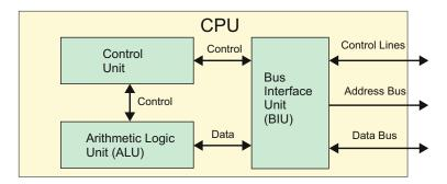
Fig. 15.2. Block diagram of a CPU.
