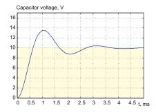
**Problem 7.101.** Capacitor voltage is measured in a series RLC circuit as shown in the figure to the previous problem. Given  $R = 2\Omega$ , estimate circuit inductance L and circuit capacitance C.
