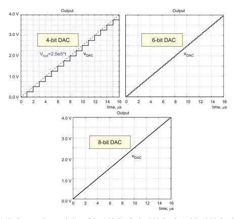
Fig. 14.17. Comparative resolution of the 4-bit DAC, the 6-bit DAC, and the 8-bit DAC. In all three cases, the full-scale output voltage range (4 V) is the same. The linear time dependence,  $v_{\rm out}(t) = 2.5 \times 10^5 t$  (V), over the time interval from 0 to 16  $\mu$ s is approximated.
