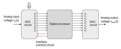
Fig. 14.20. Place of the ADC in the DSP block diagram.
