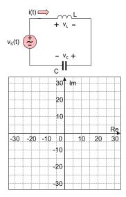
**Problem 10.4.** For a series ideal LC circuit shown in the figure below, the voltage source has the form  $v_{\rm S}(t) = V_{\rm m} \cos \omega t$ . Given  $V_{\rm m} = 5$  V, L = 1 mH,  $C = 0.5 \mu \rm F$ :
