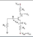
$$V_C = V_{CC} - \beta R_C I_B, I_B = \frac{V_{CC} - 0.7 \text{ V}}{R_B + (\beta + 1)R_E}$$
