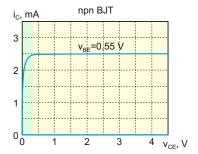
**Problem 17.12.** Using the Ebers-Moll transistor model, express the collector current  $i_{\rm C}$  in terms of the base current  $i_{\rm B}$  when the voltage across the transistor is exactly zero, i.e., when  $v_{\rm CE}=0$ .
