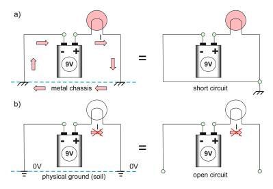
Fig. 2.38. (a) The return current path for the chassis ground is metal; it can be replaced by a wire. (b) There is no current return path, since soil (dry or wet) is a very poor conductor. The circuit is therefore open and not functioning.
