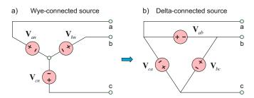
Fig. 11.28. Wye-connected source versus delta-connected source.
