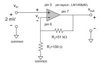
**Problem 5.26.** Determine the output voltage of the ideal operational amplifier shown in the figure. The amplifier is driven by a  $\pm 10$ -V dual power supply.
