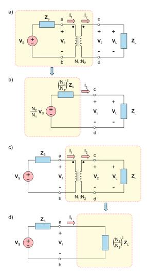
Fig. 12.6. (a) A source circuit and a load circuit connected to a transformer. (b) Equivalent circuit of the source with the transformer *when looking from the load*. (c) The same as (a). (d) Equivalent circuit of the load with the transformer *when looking from the source*.
