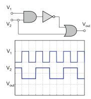
**Problem 13.57.** Given the logic circuit and the input waveforms in the following figure, draw the output waveform on the same figure. *Hint:* Construct the truth table of the logic circuit first.
