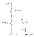
**Problem 16.21.** Assuming the ideal-diode model, find current I for the circuit shown in the figure below.
