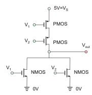
Fig. 13.21. CMOS NOR logic gate.
