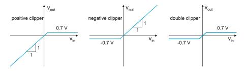
Fig. 16.35. Transfer characteristics of diode clipper circuits.
