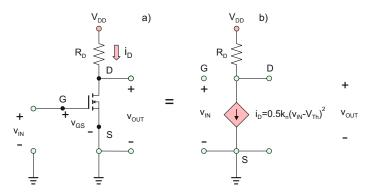
Fig. 18.27. MOSFET common-source amplifier model.
