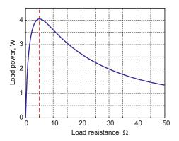
Fig. 4.18. Load power as a function of the load resistance for fixed  $V_T = 9$  V,  $R_T = 5$   $\Omega$ .
