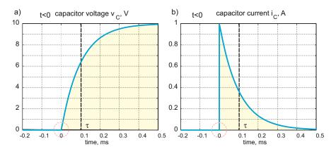
Fig. 7.8. Voltage/current plots for charging a 10- $\mu$ F capacitor in series with a 10- $\Omega$  resistor. We again observe continuity of the capacitor voltage (the "capacitor inertia").
