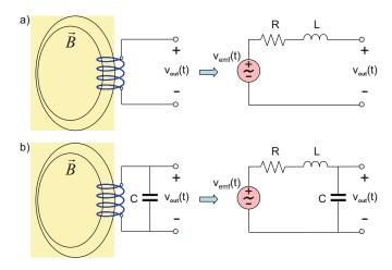
Fig. 10.19. (a) Receiver coil and (b) receiver coil with capacitance to increase the open-circuit voltage.
