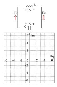
**Problem 10.3.** For a series ideal LC circuit shown in the figure below, the voltage source has the form  $v_{\rm S}(t) = V_{\rm m}\cos\omega t$ . Given  $V_{\rm m} = 5$  V, L = 0.5 mH, C = 1  $\mu$ F:
