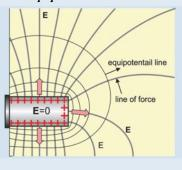
*Within conductor(s) with applied voltage:*
