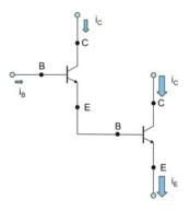
**Problem 17.7.** An npn-junction transistor in the active region at room temperature of 25 °C has  $v_{\rm BE} = 0.5 \, \rm V$ ,  $I_{\rm S} = 10^{-13} \, \rm A$ , and the base current of 0.3  $\mu A$ . Find collector current, emitter current, common-emitter current gain, and common-base current gain. Show units.
