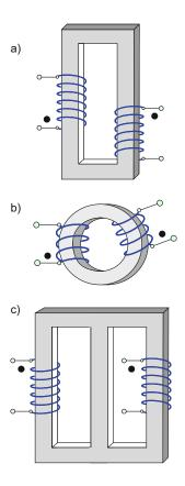
**Problem 12.3.** For the circuit shown in the following figure, determine voltage  $v_2(t)$  if  $v(t) = 100\cos\omega t$  [V] using Faraday's law of induction. Count the number of turns. Assume no flux leakage.
