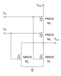
**Problem 18.38.** For a logic gate shown in the figure that follows, construct the truth table in the form of Table 18.7 and determine the output gate resistance for *every* input voltage combination. Assume  $V_{\rm DD} > V_{\rm Th}$  for the NMOS transistor and  $V_{\rm DD} > |V_{\rm Th}|$  for the PMOS transistor. Label turn-on resistances of  $M_{1,2,3,4,5,6}$  as  $r_{\rm DS1,2,3,4,5,6}$ .
