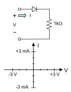
**Problem 16.34.** Sketch *I* versus *V* to scale for the circuit shown in the figure using:
