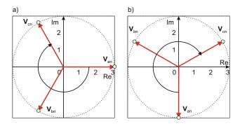
Fig. 11.15. (a) Phasor diagram for the phase sequence 0,  $+120^{\circ}$ ,  $-120^{\circ}$  and (b) phasor diagram for individual phase voltages from Eq. (11.42). Both three-phase sources are equivalent.
