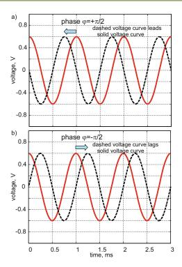
Fig. 8.2. Phase-shifted AC voltages  $v(t) = 0.6 \cos(2\pi 1000t \pm \pi/2)$  [V] versus the zero-phase voltage  $v(t) = 0.6 \cos(2\pi 1000t)$  [V] shown by a *solid curve*. In Fig. 8.2a the *dashed* voltage leads the base signal, whereas in Fig. 8.2b it lags the base signal.
