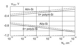
Fig. 18.6. Work function difference  $\psi_{GS}$  as a function of body doping for gate electrodes of polysilicon and aluminum, respectively, on a p-Si body of an NMOS transistor.
