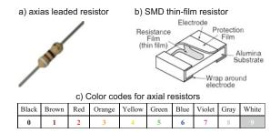
Fig. 2.7. (a) A leaded axial resistor, (b) a thin-film resistor, and (c) color codes for leaded resistors.
