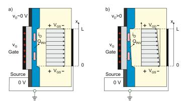
Fig. 18.12. Voltage distribution across the channel in the triode region. The linear charge and voltage profiles in Fig. 18.12b are an approximation.
