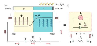
Fig. 4.23. (a) Simplified physical composition of the solar cell in the form of a pn-junction—a semiconductor diode. (b) Simplified (lossless single-diode) equivalent circuit.
