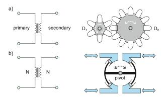
Fig. 12.5. Analogies for a transformer.
