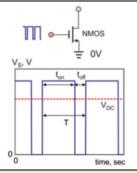
Period (sec)  $T = t_{on} + t_{off}$ Frequency (Hz) f = 1/T
