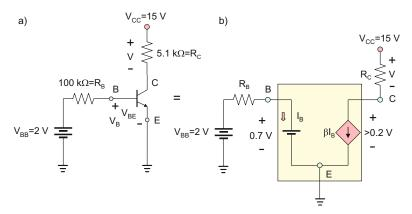
Fig. 17.16. Transistor circuit solved using the method of assumed states.
