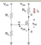
Eliminates the need in the second voltage supply ( $V_{\rm GS}$ )
