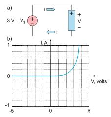
**Problem 2.31.** Plot to scale the *v-i* characteristic of the practical voltage source shown in the following figure.
