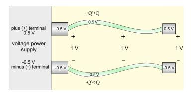
Fig. 1.3. Voltage source from Fig. 1.2 with two wires connected. There is still no current flow.
