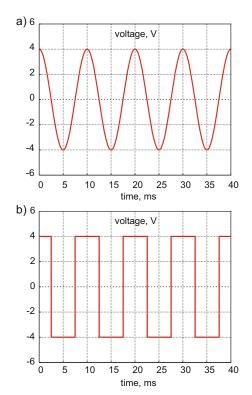
which signal delivers more average power into a resistive load? The periodic voltage on the top graph is the cosine function. Explain your answer and provide an analytical proof (find the *rms* voltages and the average power in every case).
