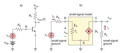
Fig. 17.36. Base-bias amplifier circuit and its small-signal model.
