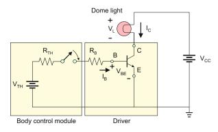
Fig. 17.30. Automotive dome light application.
