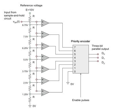
Fig. 14.26. A 3-bit flash ADC.
