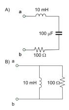
**Problem 11.23.** Determine the resistance and the reactance of the circuit block (the load) shown in the figure in terms of R, L, and C in a general form. The AC angular frequency is  $\omega$ .
