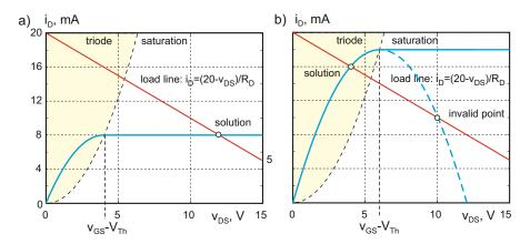
Fig. 18.23. Graphical representation of the solution for the DC circuit in Fig. 18.22 and intersection of the load line with the  $v_{\rm DS}$ — $i_{\rm D}$  curve. (a) NMOS transistor in saturation and (b) NMOS transistor in triode region.
