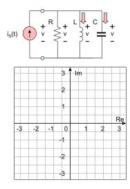
**Problem 10.19.** Determine the bandwidth, *B*, of the parallel resonant RLC circuit with the resonant frequency of 0.5 MHz and a *Q*-factor of 50.
