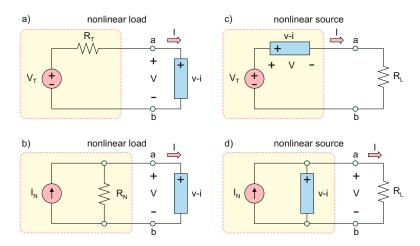
Fig. 4.20. Four basic nonlinear circuits.
