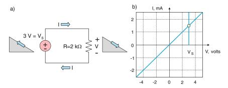
Fig. 2.19. Electric circuit solution in graphical form.
