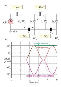
Fig. 16.31. Voltage quadrupler diode circuit and the corresponding voltage waveforms. The steady-state values of the capacitor voltages are shown in the *boxes*.
