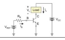
Load current is controlled by  $V_{\text{REF}}$  ( $\beta$ -dependent)
