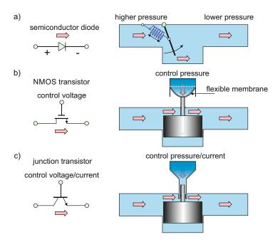
Fig. 1.11. Analogies for semiconductor circuit components.
