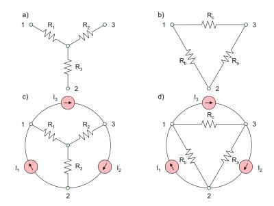
Fig. 3.27. (a) Y (wye) and (b)  $\Delta$  (delta) networks; (c) and (d) applying the superposition theorem to establish network equivalence.
