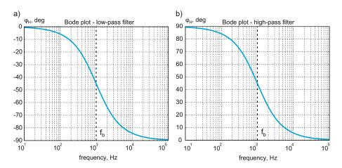
Fig. 9.6. Comparison of the phase Bode plots for (a) the low-pass-filter and (b) for the high-pass filter with the same break frequency  $f_b = 1$  kHz. Both plots are identical to within a phase shift.
