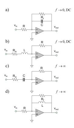
**Problem 6.55.** For two circuits shown in the figure that follows, obtain an analytical expression for the output voltage as a function of time and circuit parameters when the input voltage has the form  $v_{\rm in}(t) = 1 \exp(-\alpha t)$  [mV].
