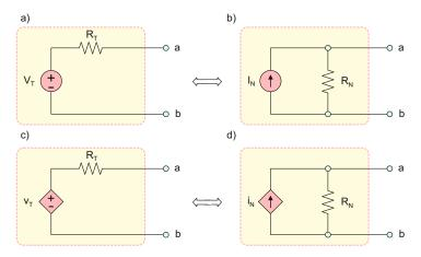
Fig. 4.8. Transformation of dependent and independent sources.
