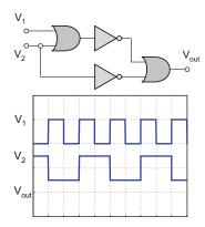
**Problem 13.58.** Given the logic circuit and the input waveforms in the following figure, draw the output waveform on the same figure. *Hint:* Construct the truth table of the logic circuit first.
