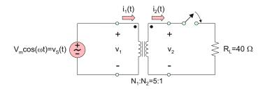
Fig. 12.4. A transformer circuit with a load and a switch.
