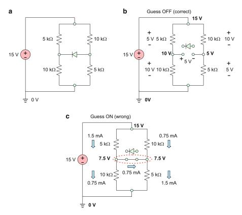
Fig. 16.11. (a) A resistor network bridged with an ideal diode. (b) Circuit analysis assuming the diode state is OFF (correct guess), leading to an open circuit. Absolute voltages versus ground are marked in *bold*. (c) Circuit analysis assuming the diode state ON (wrong guess), which is a short circuit. The absolute voltages with respect to ground are marked in *bold*.
