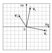
Fig. 8.8. Phasor diagram for three time-domain voltages  $v_1(t)$ ,  $v_2(t)$ ,  $v_3(t)$ . Voltage  $v_2(t)$  leads voltage  $v_1(t)$  by 90°, but lags voltage  $v_3(t)$ .
