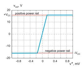
Fig. 5.2. Amplifier output voltage in the open-loop configuration. The open-loop gain is  $A_{\rm OL} = 10^5$  and the supply voltage is  $\pm 16$  V. Note that the scale for the input voltage is in mV.
