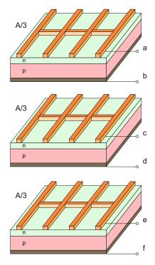
**Problem 4.23.** Individual solar cells in the figure to the previous problem are to be connected into a standard solar module. Draw the corresponding wire connections.
