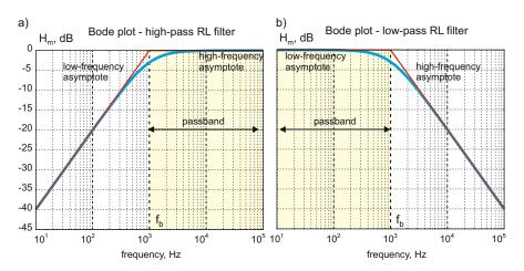
Fig. 9.10. (a) Bode plot for the amplitude transfer function of the high-pass RL filter with break frequency  $f_b = 1 \text{ kHz}$ . (b) The same Bode plot but for the low-pass RL filter.
