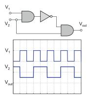
**Problem 13.59.** Given the logic circuit and the input waveforms in the following figure, draw the output waveform on the same figure. *Hint:* Construct the truth table of the logic circuit first.
