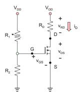
Fig. 18.25. Gate-bias NMOS transistor circuit with the voltage divider.
