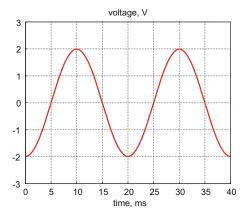
**Problem 8.9.** An AC voltage in a circuit is given by  $v(t) = 10\cos{(2\pi50t)}$  [V]. Using software of your choice, plot the voltage to scale over the time interval of two periods, i.e.,  $0 \le t \le 2T$ . Label the axes.
