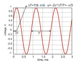
Fig. 8.3. A phase-shifted AC voltage  $v(t) = 1 \cos(2\pi 1000t - \pi/3)$  [V].
