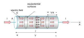
Fig. 2.5. Finding the resistance of a conducting cylinder.
