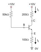
**Problem 17.37.** For the circuit shown in the figure, determine the transistor current gain  $\beta$ . Use the large-signal DC circuit model of the transistor.
