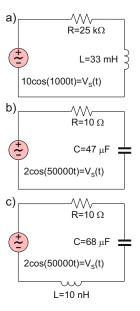
**Problem 8.43.** Repeat problem 8.42 if the AC voltage power supply in every figure is replaced by an alternating current power supply with the same frequency and amplitude of 0.5 A.
