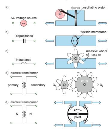
Fig. 1.10. Hydraulic analogies for alternating-current (AC) circuit elements.
