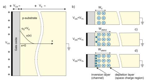
Fig. 18.5. (a) Central region of the MOSFET under an applied voltage  $v_{\rm GS}$ : the MOS capacitor. (b) to (d) Formation of the depletion and inversion layers in the substrate. The entire region close to the semiconductor surface is called the *surface space-charge region*.
