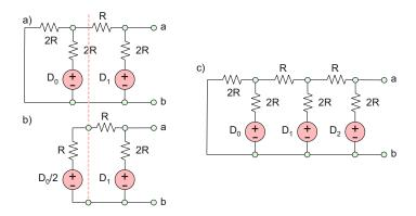
Fig. 4.14. Two-bit and three-bit *R*-2*R* ladder networks.
