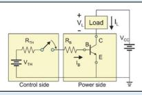
$$R_B = rac{V_{TH} - 0.7 \text{ V}}{I_B} - R_{TH}, I_B \approx 2 rac{V_{CC}}{\beta R_L}$$
