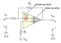
**Problem 5.71.** For two nonideal operational amplifier circuits (with the nonzero input offset voltage) shown in the figures below, determine the necessary offset voltage,  $V_{\text{off}}$ , which ensures that the output voltage,  $v_{\text{out}}$ , to the amplifier exactly follows the ideal-amplifier gain law:  $v_{\text{out}} = A_{\text{CL}}v_{\text{in}}$ . You need to express this voltage in terms of other circuit parameters that are given in figures a) and b).
