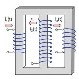
**Problem 12.11.** In Problem 12.6, determine the instantaneous stored energy of a nonideal transformer given a core centerline length of 30 cm.
