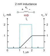
Fig. 6.16. Impressed current through an inductance (*solid curve*) and resulting voltage across the inductance (*dashed curve*).
