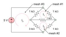
Fig. 4.5. Circuit solution using the mesh analysis. Circuits in Figs. 4.5 and 4.1 coincide.
