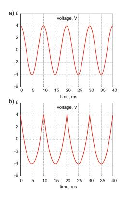
**Problem 11.13.** Of the two periodic signals shown in the figure that follows, which signal delivers more average power into a resistive load? The periodic voltage on the top graph is the cosine function. Explain your answer and provide:
