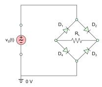
Fig. 16.24. The full-wave diode bridge rectifier: four diodes are bridged by the load resistor R<sub>L</sub>.
