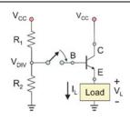
Constant-voltage source (voltage follower or voltage buffer,  $\beta$ -independent) in common collector or emitter follower configuration
