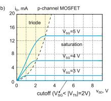
Fig. 18.14. (a) Drain current as a function of the drain-source voltage for an NMOS transistor with  $V_{\rm Th}=2~{\rm V}$  and  $k_n=3~{\rm mA/V^2}$ . (b) Drain current as a function of the source-drain voltage for a PMOS transistor with  $|V_{\rm Th}|=2~{\rm V}$  and  $k_{\rm p}=3~{\rm mA/V^2}$ .
