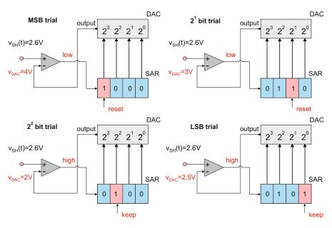
Fig. 14.28. Operation of a 4-bit successive-approximation ADC.
