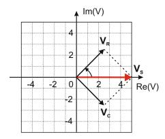
Fig. 8.15. Phasor diagram for the circuit in Fig. 8.14 and KVL in the vector form.
