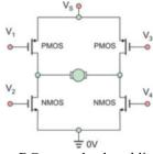
Controls a DC motor load enabling:
