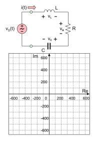
**Problem 10.8.** In the series resonant RLC circuit shown in the figure below, given  $V_m = 5 \text{ V}$ ,  $L = 30 \text{ }\mu\text{H}$ , C = 0.48 nF,  $R = 50 \text{ }\Omega$ :
