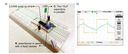
Fig. 7.22. (a) Timer circuit operation in laboratory. The square waveform is the output voltage  $v_{\text{out}}(t)$ . The curved waveform is the capacitor voltage  $v_{\text{C}}(t)$ . A variable resistance R makes it possible to visually control the oscillation frequency using an LED connected to the output through a buffer amplifier. The oscillation frequency changes from 0.5 to about 100 Hz.
