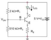
Constant-current source—the 5 V—LED drive of 20 mA (any color LED,  $\beta$ -independent)
