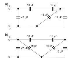
**Problem 6.12.** Find the equivalent capacitance for each circuit shown in the following figure.
