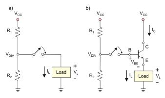
Fig. 17.25. Voltage divider circuit comparison.
