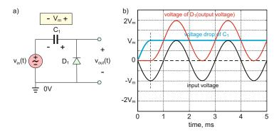
Fig. 16.29. Diode clamper circuit and the corresponding voltage waveforms. The steady-state value of the capacitor voltage is shown in the *box*.
