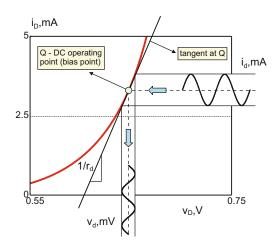
Fig. 16.16. Linearization procedure for a switching diode with  $n = 1.7, I_S = 1.1 \,\mathrm{nA}$  at 25 °C.
