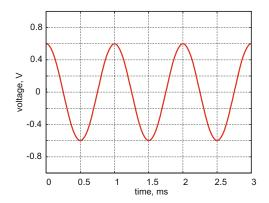
**Problem 8.4.** Repeat problem 8.2 for a harmonic voltage signal with a DC offset shown in the figure below.
