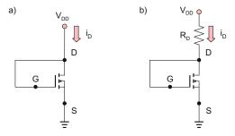
Fig. 18.24. Diode-connected MOSFET circuit with  $v_{\rm GS} = v_{\rm DS}$ .
