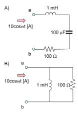
**Problem 11.20.** Determine the average power delivered to the load circuit between terminals a and b shown in the figure that follows. The AC angular frequency is 1000 rad/s.
