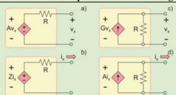
Case b):  $R_{\rm T} = R - Z$ Case c):  $R_{\rm T} = \frac{R}{1 - GR}$ Case d):  $R_{\rm T} = R(1 - A)$ Equivalent resistance may become negative
