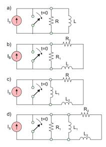
Fig. 7.24. Transient circuits with multiple resistances and inductances.
