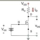
The load line:  $i_D = (V_{DD} - v_{DS})/R_D$
