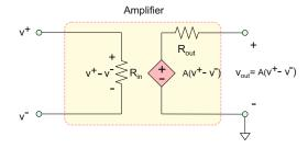
Fig. 5.4. Equivalent circuit model of an amplifier is in the shadow box as a two-port network. No load is connected. The ground of the output terminal is the common port.
