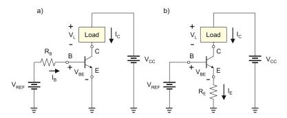
Fig. 17.23. Simple BJT configuration as constant-current sources.
