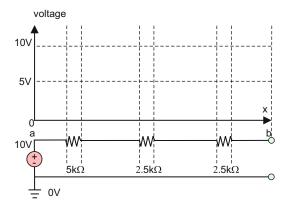
**Problem 3.41.** For the circuit shown in the following figure, use the voltage division principle to calculate  $V_1$ ,  $V_2$ ,  $V_3$ .
