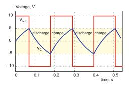
Fig. 7.21. Relaxation oscillator operation for the idealized amplifier model (amplifier hits the rails in saturation); the amplifier supply voltage is 10 V.
