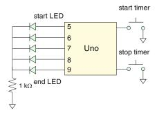
**Problem 15.56.** Write a program that turns the Arduino into a rudimentary stopwatch. The Arduino should begin "timing" after the push of a push button and then "stop" timing after a push of a different button. A sketch is shown in the following figure. *Hint:* Use some of the built-in timing features.
