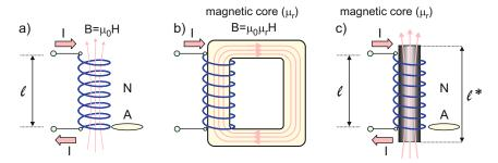
Fig. 6.11. Three types of a solenoid.
