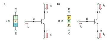
Fig. 17.9. The npn BJT and its pnp complement. We notice the collector and emitter reversal.
