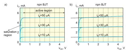
Fig. 17.8. Typical common-emitter characteristics of the npn BJT. The collector current is independent of the collector-to-emitter voltage in the active region in (a). (b) shows a more accurate representation which includes the *Early effect*.
