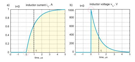
Fig. 7.13. Voltage/current plots for "charging" the 1-mH inductor in parallel with the 1-k $\Omega$  resistor.
