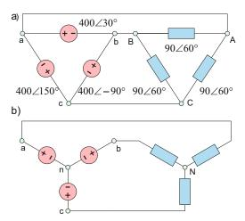
Problem 11.54. A balanced delta-delta system shown in the figure below operates at 50 Hz. The phase voltages of the delta source,  $V_{ab}$ ,  $V_{bc}$ ,  $V_{ca}$ , have the amplitudes of  $V_{m} = 563.4$  V each. Every phase impedance is a 0.21 H inductance in series with a 38-Ω resistance:
