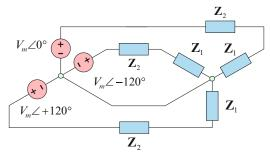
**Problem 11.41.** Prove that Eq. (11.28) of this chapter for line voltages also holds for the negative phase sequence to within the substitution  $30^{\circ} \rightarrow -30^{\circ}$ .
