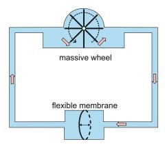
Fig. 10.2. Self-oscillating mechanical counterpart of the LC circuit shown in Fig. 10.1.
