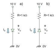
**Problem 16.18.** Using the ideal-diode model, you need to design a circuit for the diode temperature sensor described in Problem 16.10.
