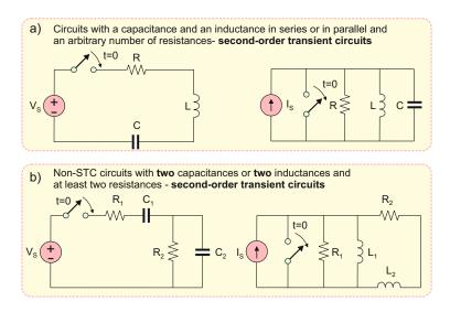
Fig. 7.29. Classification of second-order transient circuits.
