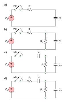
Fig. 7.23. Transient circuits with multiple resistances and capacitances.
