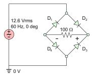
*Note:* The voltage source shown represents the output of a typical step-down transform and is given in *rms*.
