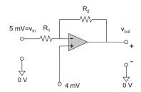
**Problem 5.67.** In the previous problem, denote the terminal voltage of 4 mV by  $V_{\rm off}$ , the input voltage of 5 mV by  $v_{\rm in}$ , the output voltage by  $v_{\rm out}$ , and the amplifier gain by  $A_{\rm CL}$ . Derive an analytical formula that determines  $V_{\rm off}$  in terms of  $v_{\rm in}$  given that the output voltage to the amplifier is exactly zero.
