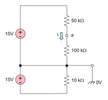
**Problem 3.68.** Determine the absolute voltage (versus chassis ground) and the current i at the circuit point a.
