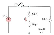
**Problem 6.39.** Find current I in the circuit shown in the following figure at  $t \to \infty$ , in the DC steady state. The switch closes at t = 0.
