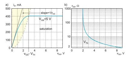
Fig. 18.18. MOSFET turn-on resistance  $r_{\rm DS}$  and its dependence on gate-source voltage for a 2 N7000 NMOS device.
