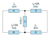
**Problem 3.7.** Find a relation between currents  $i_C$ ,  $i_E$  for the circuit shown in the following figure. Does the problem have a unique solution?
