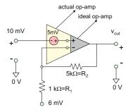
**Problem 5.69.** Solve the previous problem with the offset voltage in the feedback loop changed from 6 mV to 5 mV.
