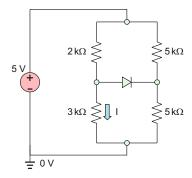
**Problem 16.23.** For the circuit shown in the figure below, determine circuit current I, assuming that the diode is ideal. The ground path is simultaneously the current return path.
