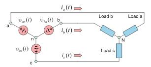
Fig. 11.24. Three-phase balanced wye-wye circuit in the time domain. Three individual loads are identical. Each of them is characterized by the impedance  $\mathbf{Z} = Z \angle \theta$  in the frequency domain.
