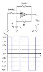
Sketch to scale the capacitor voltage,  $v_{\rm C}$ , as a function of time. Assume that  $v_{\rm C}(t=0)=0$ . Assume the ideal amplifier model. The specific values of R and C do not matter; they are already included in the time scale.
