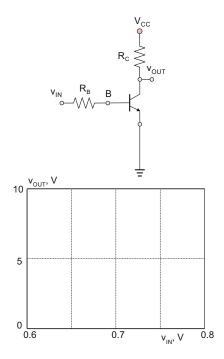
**Problem 17.53.** Determine small-signal baseemitter resistance  $r_{\pi}$  of a BJT at room temperature of 25 °C given that
