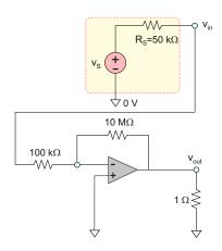
**Problem 5.58.** An amplifier circuit is needed with the closed-loop gain  $A_{\rm CL} = +1000$ . The input resistance (impedance) to the circuit should be 5 k $\Omega$ . Present two alternative circuit diagrams and specify the necessary resistor values. The first circuit must use inverting amplifiers and the second circuit-non-inverting amplifiers.
