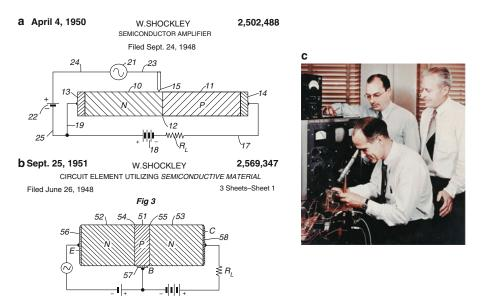
Fig. 17.10. (a) An early concept of a semiconductor amplifier on the basis of a single pn-junction; (b) evolution of the pn-junction concept resulted in the invention of the bipolar junction transistor. Both figures are from the original patents. (c) William Bradford Shockley (seating), John Bardeen and Walter Brattain Bell Labs, June 1948.
