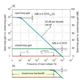
Fig. 9.13. Closed-loop AC gain  $A_{\rm CL}(f)$  (lower curve) versus open-loop AC gain  $A_{\rm OL}(f)$  (upper curve) for an inverting amplifier with  $A_{\rm OL}(0) = 10^5$  and  $1 + R_2/R_1 = 10$  (the amplifier DC gain is -9).
