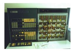
Fig. 14.10. An analog computer from Electronic Associates, Inc. West Long Branch, New Jersey, with 156 individual amplifiers (Analog Computer Museum by Doug Coward).
