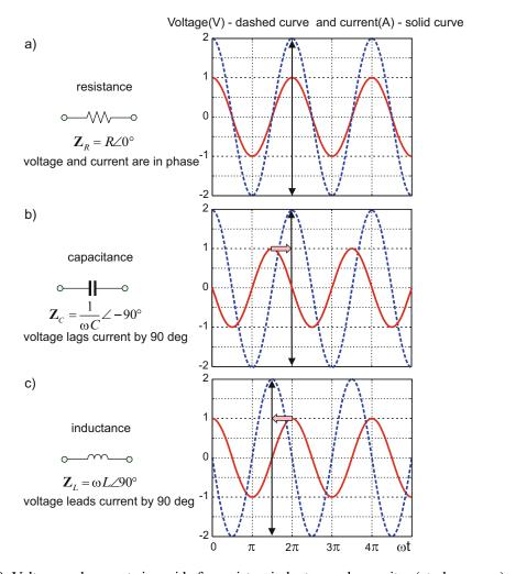
Fig. 8.10. Voltage and current sinusoids for resistor, inductor, and capacitor (at phase zero).
