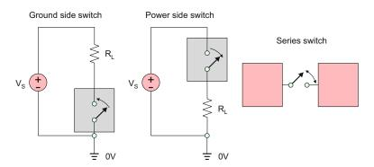
Fig. 13.2. Switch positions in a circuit.
