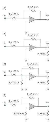
**Problem 5.36.** An inverting amplifier that achieves high-gain magnitude with a smaller range of resistance values is shown in the figure below. Find its output voltage  $v_{\text{out}}$  vs. ground (or common port) and the resulting amplifier gain.
