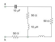
**Problem 6.43.** Determine the equivalent resistance between terminals a and b for the circuit shown in the following figure in the DC steady state.
