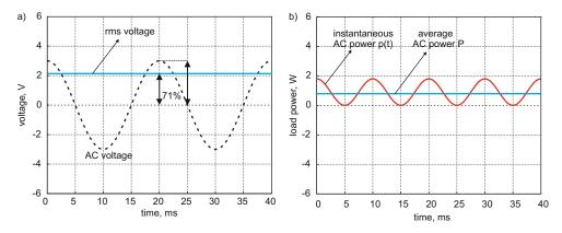
Fig. 11.2. (a) Load voltage  $v(t) = 3\cos(2\pi 50t)$  [V] (dotted line) and its rms DC voltage, which delivers the same power into the load and (b) instantaneous power and the average power for the load voltage  $v(t) = 3\cos(2\pi 50t)$  [V].
