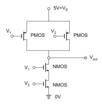
Fig. 13.25. CMOS NAND logic gate.
