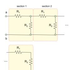
*Hint:* For the semi-infinite ladder network in the previous figure, the equivalent resistance  $R_{\rm eq}$  will not change after adding a new section up front as shown in the figure that follows:
