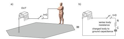
Fig 6.2. Equivalent circuit for understanding ESD and its effect on a device under test (DUT).
