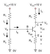
Fig. 17.20. Four-resistor bias circuit.
