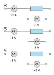
**Problem 2.29.** The figure that follows shows a circuit with a passive nonlinear circuit element shown by a rectangle.
