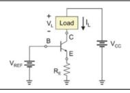
Load current is controlled by  $V_{REF}$  ( $\beta$ -independent)
