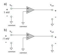
**Problem 5.33.** Each of the circuits shown in the figures below employs negative feedback. Find the output voltage  $v_{\text{out}}$  vs. ground (or common). *Hint:* The ground symbol in an amplifier circuit usually has the *same* meaning as the common port.
