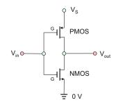
Problem 13.6. For the circuit shown in the figure below,  $V_{\rm S} = 2.5$  V and  $V_{\rm Tn} = |V_{\rm Tp}| =$ 0.5 V (0.25-µm CMOS process). Determine the output voltage  $V_{\text{out}}$  when:
