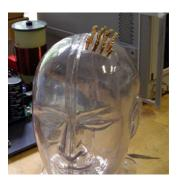
Fig. 12.21. An array of coupled inductors (small coils) located on top of a human-head phantom. This hypothetic setup was tested for applications related to brain stimulation.
