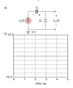
**Problem 16.66.** In the clamper circuit shown in the figure for Problem 16.65,  $v_{\rm in}(t) = V_{\rm m} - V_{\rm m} \sin \omega t$  and  $V_{\rm m} = 4 \, \rm V$ . The wave period is 2 ms.
