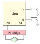
The circuitry should use two push button switches to choose the direction.
