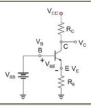
$$V_C = V_{CC} - \beta R_C I_B, I_B = \frac{V_{BB} - 0.7 \text{ V}}{(\beta + 1)R_E}$$
