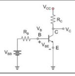
$$V_C = V_{CC} - \beta R_C I_B$$
