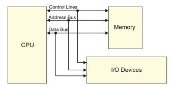
Fig. 15.1. Architecture of a generic computer.
