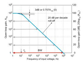
Fig. 9.11. Bode plot of the open-loop gain magnitude for the LM741-type amplifier IC. Note the logarithmic scale on the *left* and the corresponding scale in dB on the *right*. The frequency bandwidth given by the break frequency  $f_b$  is only 10 Hz.
