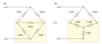
Fig. 3.28. Network simplification using  $\Delta$  to Y transformations.
