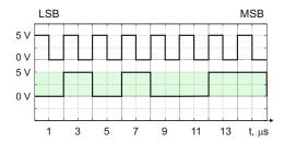
Fig. 14.9. Timing diagram for a binary bit steam.
