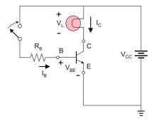
**Problem 17.49.** For the circuit shown in the figure below,  $V_{\rm CC}=12\,{\rm V}$ , and the bulb turn on resistance is 40  $\Omega$ . Assume the minimum value  $\beta=30$ .
