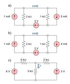
**Problem 4.45.** Solve the circuits shown in the following figure—determine unknown voltage V or current I (show units). You can use any of the methods studied in class:
