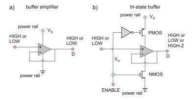
Fig. 14.12. Concept of a tri-state buffer.
