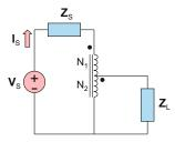
**Problem 12.36.** Find the equivalent input impedance,  $\mathbf{Z}_{in}$ , for two autotransformer circuits shown in the following figure.
