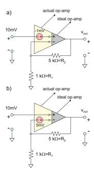
**Problem 5.63.** Determine the output voltage to nonideal operational amplifier circuits (with nonzero input currents) shown in the figures below. The input terminal is connected directly to the common terminal (grounded). The strength of every bias current source is 100 nA. *Hint:* The upper bias current source does not contribute to the solution.
