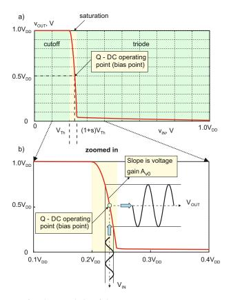
Fig. 18.28. Voltage transfer characteristic of the MOSFET common-source amplifier (a) and the amplification principle (b). The output sinusoidal signal indicates no distortion, which is a simplification. Circuit parameters are those from Exercise 18.14.
