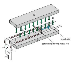
Fig. 7.4. An electromagnetic accelerator based on the Lorentz force effect in the magnetic field created by two permanent magnets and the capacitor discharge current.
