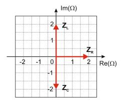
Fig. 8.12. Complex impedances displayed in the phasor diagram.
