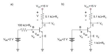
Fig. 17.19. Two candidates for the transistor bias circuit.
