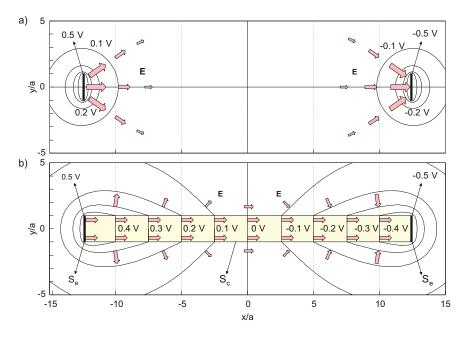
Fig. 1.6. (a) Two electrodes subject to  $\pm 0.5$  V in free space; (b) the same electrodes but with a conducting cylinder between them. Equipotential lines and electric field vectors are shown.
