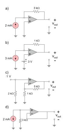
**Problem 5.34.** Each of the circuits shown in the figures below employs negative feedback. Find the output voltage  $V_{out}$  vs. ground (or common). *Hint:* The ground symbol in the amplifier circuit usually has the same meaning as the common port.
