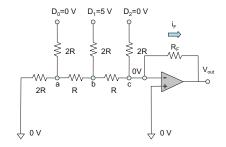
**Problem 14.38.** By solving the amplifier circuit, determine the output voltage of the 4-bit R/2R ladder DAC in Fig. 14.18 given that  $D_3 = 0$  V,  $D_2 = 5$  V,  $D_1 = 0$  V,  $D_0 = 0$  V.
