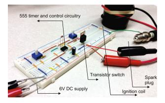
Fig. 7.16. A constructed ignition system.
