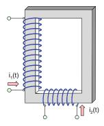
**Problem 12.8.** For the circuit shown in the following figure, establish the relation between currents  $i_1(t)$ ,  $i_2(t)$ , and  $i_3(t)$ . Assume an ideal magnetic core. Count the number of turns.
