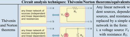
Any linear network with independent sources, dependent linear sources, and resistances can be replaced by a simple equivalent network in the form:
