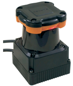
Fig. 6.6. A scanning laser range finder. The sensor has a rotating assembly that emits pulses of infra-red laser light and measures the time taken for the reflection to return. This sensor has a maximum range of 30 m and an angular range of 270 deg. Angular resolution is 0.25 deg and the sensor makes 40 scans per second (Courtesy of Hokuyo Automatic Co. Ltd.)
