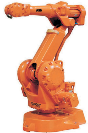
Fig. 1.3. A modern six-axis robot from ABB that would be used for factory automation. This type of robot is a technological descendant of the Unimate shown in Fig. 1.2
