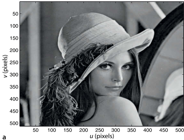
Fig. 12.12. Smoothing. a Original image; b smoothed with a 21 \times 21 averaging kernel; c smoothed with a 31 \times 31 Gaussian G(\sigma=5) kernel
